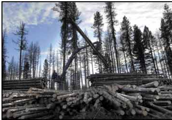
A Pyramid Mountain Lumber Co. forwarder picks up and stacks logs Tuesday as part of a thinning project in the Swan Lake Ranger District of the Flathead National Forest.
